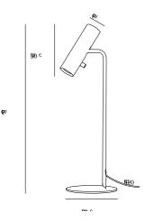
Voltage (V): 230 Volt IP degree: IP20 Maximum bulb wattage (W): 8W Class (Class 1, Class 2, Class 3): Class 2 (Double isolated) Bulb base: GU10 Dimmerable: Yes with compatible
