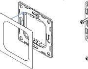
Method 1:Stick 3M glue on the back of the bracket and then stick to the wall the bracket to the wall
