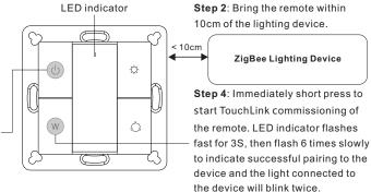
Note: 1) Directly TouchLink (both not added to a ZigBee network), each remote can link with 30 devices.
