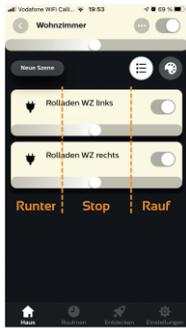
Both actuators are dimmed ~50%. They are thus between 30% and 70% which stops the actuator (motor).
